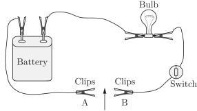
Insert sample to be tested Metals are good conductors of electricity
